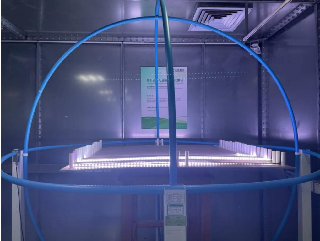
Photograph 2: Set-up for Radiated Electromagnetic Disturbances (30MHz-1000MHz)
