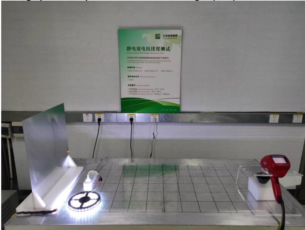
Photograph 7: Set-up for Electrostatic Discharges (ESD)
